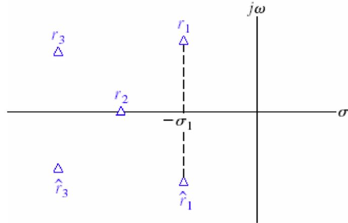
One method of determining the relative stability of each root is to use an axis shift in the s-domain and then use the Routh array as shown in Example 6.6 of the text.
