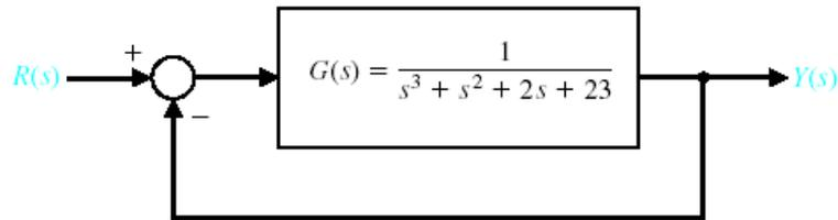
Closed-loop control system with  $T(s) = Y(s)/R(s) = 1/(s^3 + s^2 + 2s + 23)$
