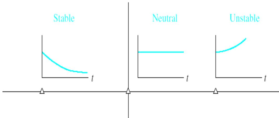
A necessary and sufficient condition for a feedback system to be stable is that all the poles of the system transfer function have negative real parts.
